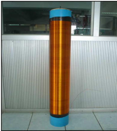
Figure 4 :High Voltage Winding which winding with the 6 inches PVC Tube
